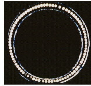
Figure 2: Tip of the laser sheath with the optical fibers circumferentially arranged around the tip
