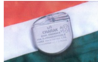
Figure 3: Charak: DDD, multi-programmable pacemaker
