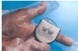
Figure 2: Pinnacle: VVI, multi- programmable pacemaker
