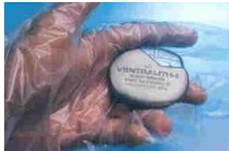
Figure 1: Ventralith-I: VVI Non- Programmable Pacemaker
